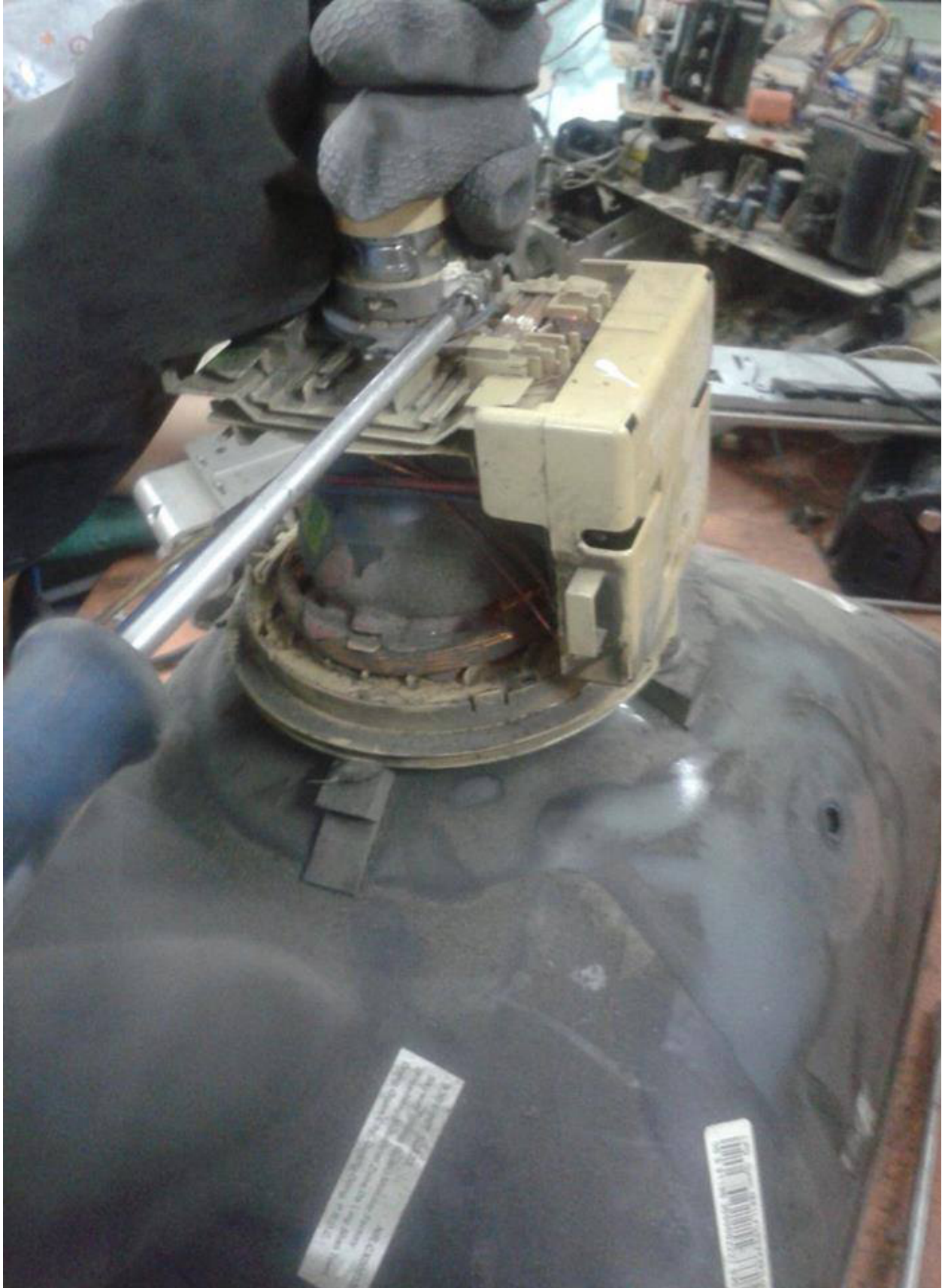
Dismantling the CRT Components including PCB
