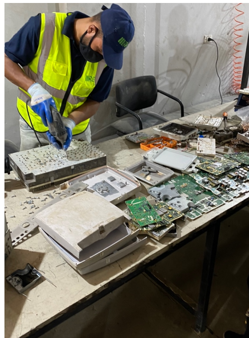
Figure 3: On the left three workers are shown dismantling old VHS cassettes and e-waste equipment. On the right a worker is depicted dismantling a PCB from communication tower equipment.
