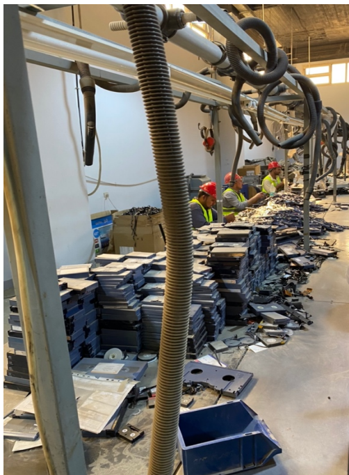
Figure 3: On the left three workers are shown dismantling old VHS cassettes and e-waste equipment. On the right a worker is depicted dismantling a PCB from communication tower equipment.
