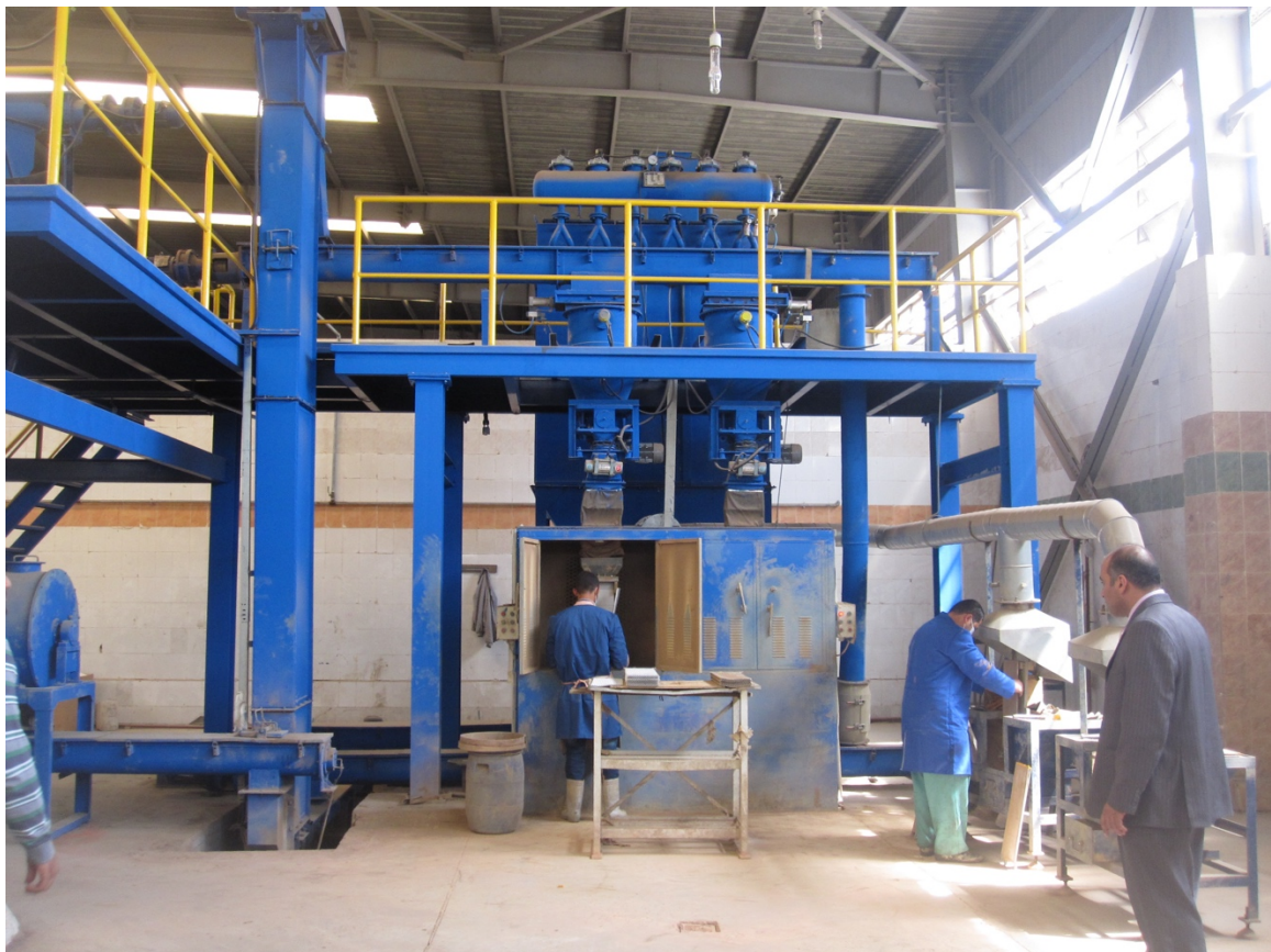
Figure 12: Lead plates separation at EIMotahda Facility
