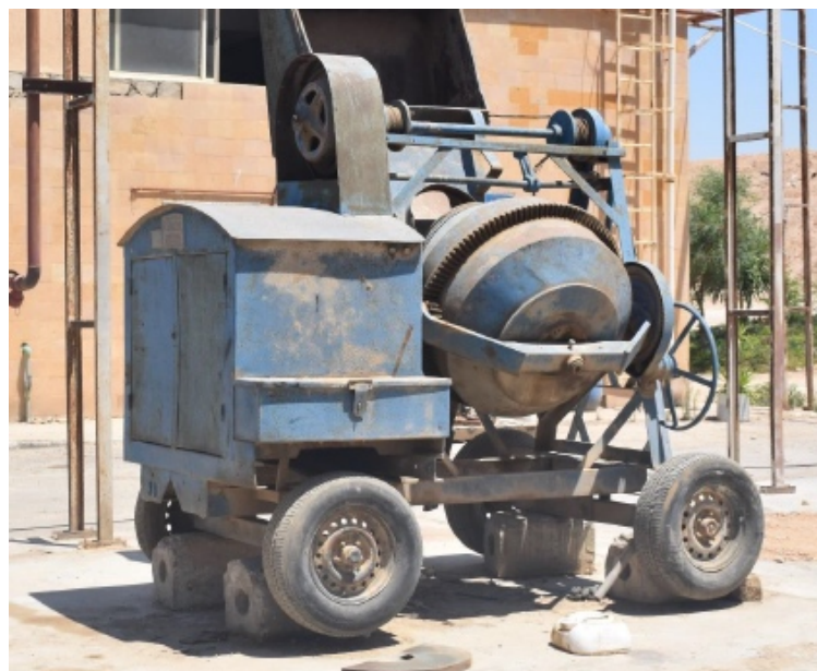
Figure 16: Solidification unit according to site visit to Al-Nasreya landfill.
