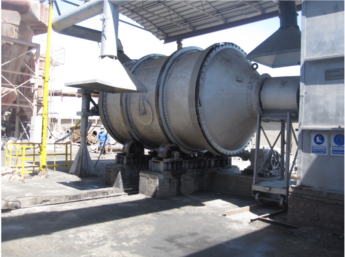
Figure 13: Rotary furnace for lead smelting at ElMotahda Facility
