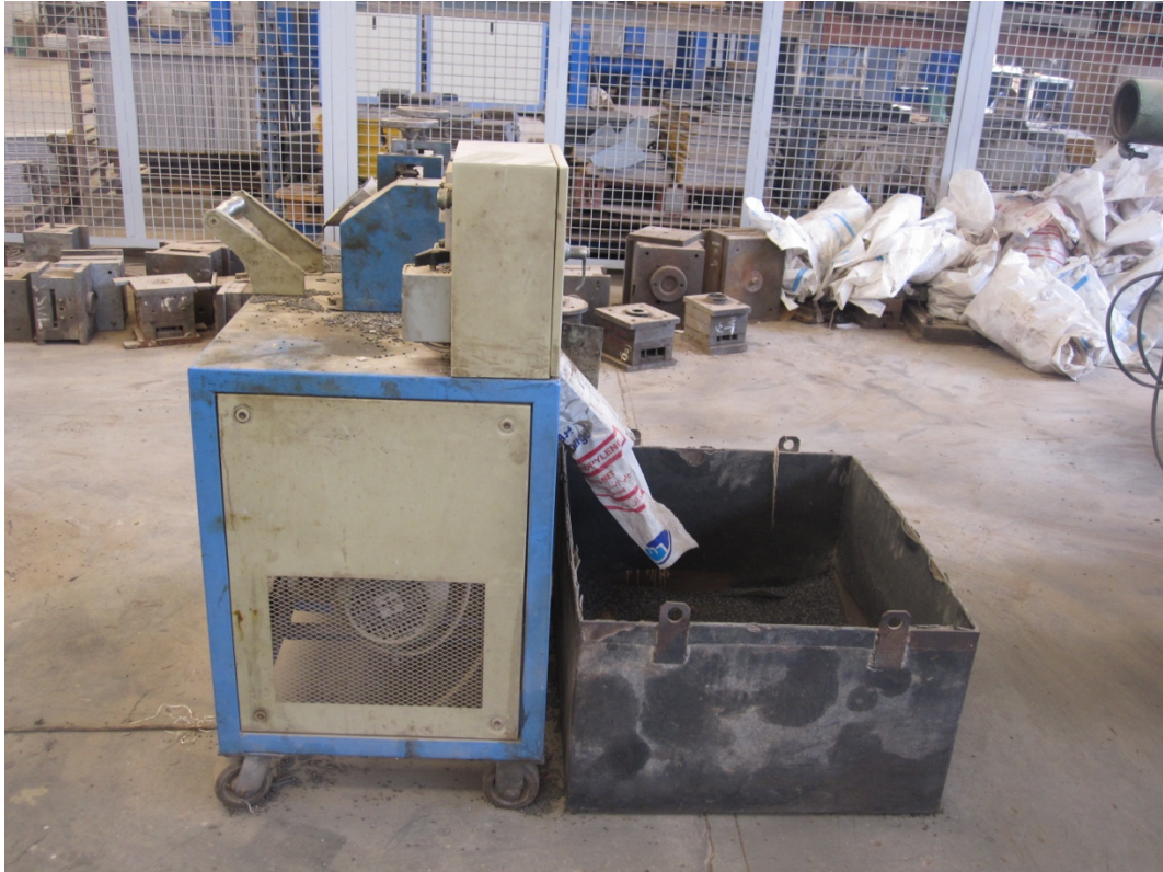
Figure 15: Plastic crushing for recycling at ElMotahda Facility
